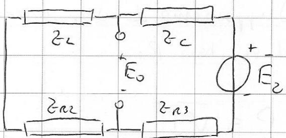
$$\bar{E}_o = \bar{E}_1 \cdot \frac{\bar{Z}_{R3} + \bar{Z}_c}{\bar{Z}_{R2} + \bar{Z}_{R3} + \bar{Z}_L + \bar{Z}_c} + \bar{E}_2 \cdot \frac{\bar{Z}_{R2} + \bar{Z}_L}{\bar{Z}_{R2} + \bar{Z}_{R3} + \bar{Z}_L + \bar{Z}_c} = -6 + 13j$$
