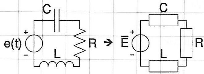
$$\begin{aligned} \bar{E} &= 160 \\ Z_R &= 8 \\ Z_C &= -j \quad \text{perche in} \\ Z_L &= j \quad \text{perche non} \end{aligned}$$
