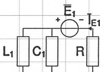
$$\bar{I}_{E1} = \bar{I}_R = \frac{\bar{E}_1}{Z_R + Z_{L1} // Z_{C1}} = 36 + 12j$$
