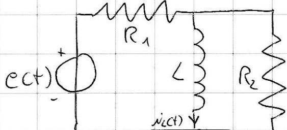
$$e(t) = \begin{cases} 0 \text{ V}, & t < 0 \\ 8 \text{ V}, & 0 < t < T \\ 0 \text{ V}, & t > T \end{cases}$$
