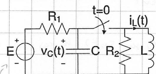
$$\begin{aligned} E &= 90 \text{ V} \\ R_1 &= 3 \Omega \\ R_2 &= 6 \Omega \\ L &= 2.5 \text{ mH} \\ C &= 0.1 \text{ mF} \end{aligned}$$
