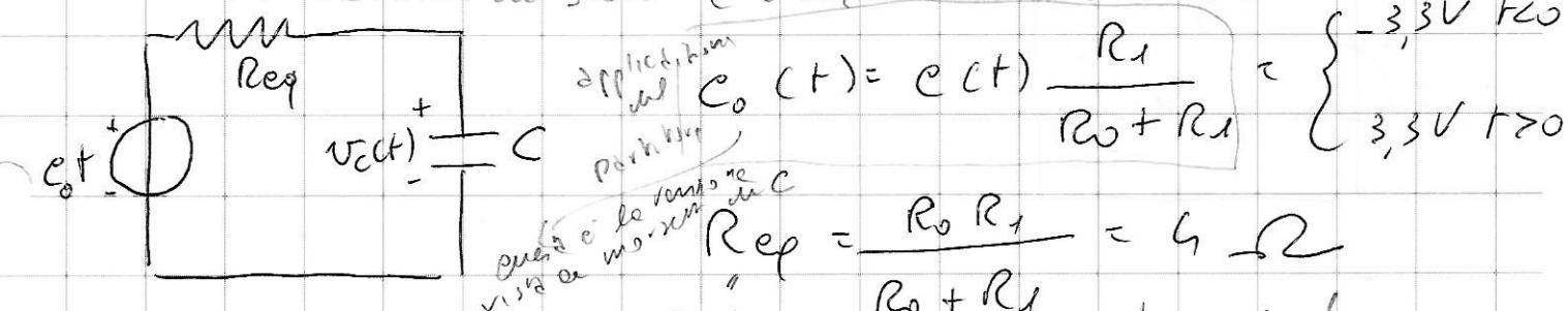
$$V_{th} = e(t) \frac{R_1}{R_0 + R_1} = 3,3V$$
