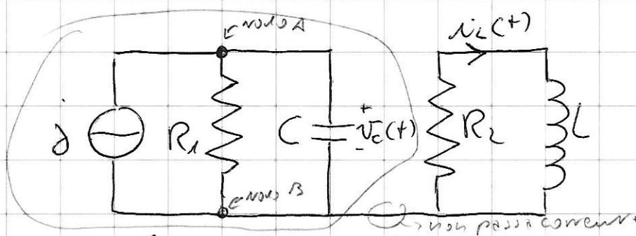
$$\left\{ \begin{array}{l} \frac{V_c}{R_1} + i_c = J \quad \text{LKCC} \\ i_c = C \frac{dV_c}{dt} \quad \text{caratteristica del condensatore} \end{array} \right.$$
