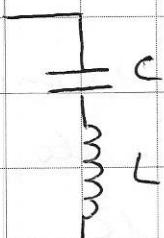
$$\text{se } LC\omega^2 = 1 \text{ ovvero } \omega = \frac{1}{\sqrt{LC}}$$
