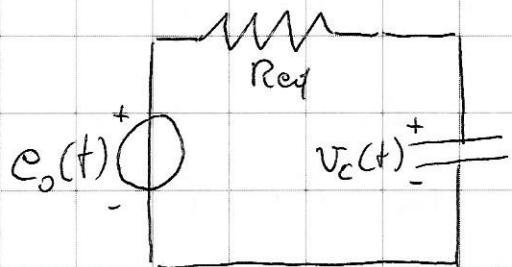
$$e_o(t) = e(t) \cdot \frac{R_1}{R_0 + R_1} = \begin{cases} -3,3V & t < 0 \\ 3,3V & t > 0 \end{cases}$$
