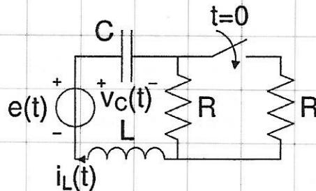
$$\begin{aligned} e(t) &= 160 \cos(500t) \text{ V} \\ R &= 8 \Omega \\ C &= 2 \text{ mF} \\ L &= 2 \text{ mH} \end{aligned}$$
