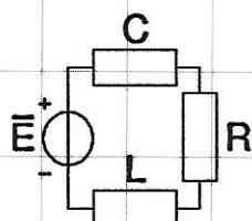
$$\begin{aligned} \bar{I}_L &= \frac{\bar{E}}{Z_R + Z_L + Z_C} = 20 \\ \bar{V}_C &= Z_C \bar{I}_L = -20j \end{aligned}$$
