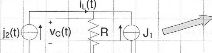
$$v_{cp}(t) = R(J_1 + j_2) = 270 \text{ V}$$
