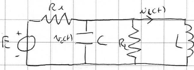
$$\left\{ \begin{array}{l} E - R_1 i_1 - V_C = 0 \\ V_C = R_2 i_2 = L \frac{dV_C}{dt} \\ i_1 - C \frac{dV_C}{dt} - i_2 - i_L = 0 \end{array} \right.$$
