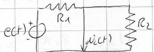
$$0 + \frac{R_1 R_2}{(R_1 + R_2)L} A = \frac{R_1}{(R_1 + R_2)} \cdot e(t)$$
