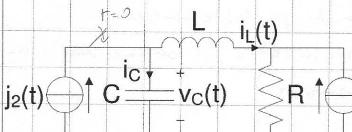
$$\begin{aligned} J_1 &= 20 \text{ A} \\ j_2(t) &= \begin{cases} 0 \text{ A}, & t < 0 \\ 7 \text{ A}, & t > 0 \end{cases} \\ R &= 10 \Omega \\ L &= 10 \text{ mH} \\ C &= 625 \mu\text{F} \end{aligned}$$
