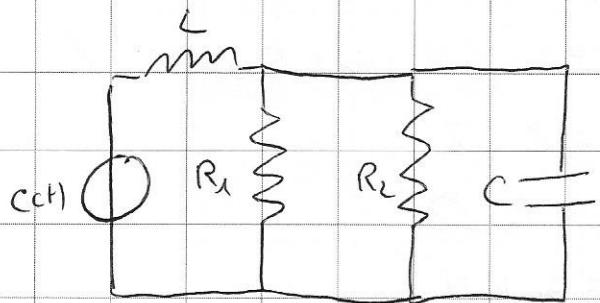
$$R_{12} = R_1 \parallel R_2 = 1/R$$
