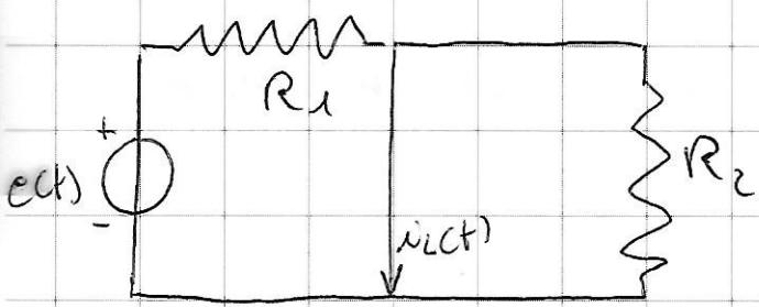
$$i_L(t) = \frac{e(t)}{R_2} = 0 \text{ A} \quad t < 0$$
